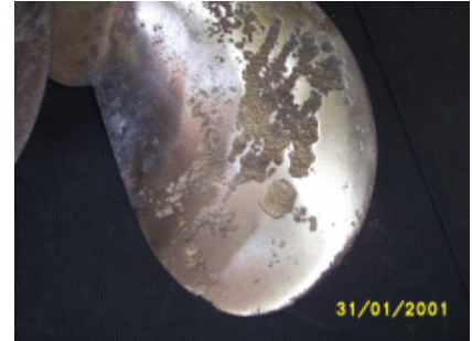
Closeup on the effects of Electrolysis Corrosion. (Heavy pitting and metal loss.)
